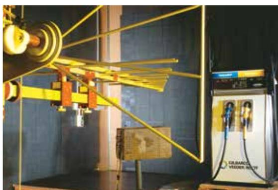
*Petrol bowsers need to be examined for compliance to specifications. One of the tests is to ensure that their measurements are not susceptible to electromagnetic interference.*
