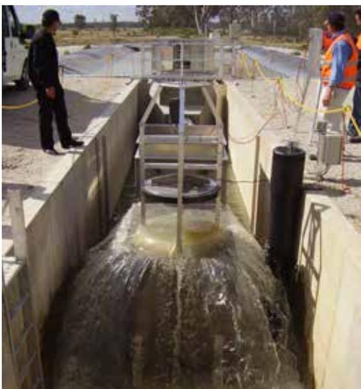
*A new irrigation metering system being tested. Together with the water industry, NMI has developed a new irrigation meter standard to help manufacturers and users ensure consumption of irrigation water is measured accurately.*
