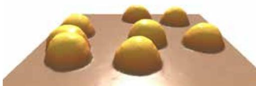
*An image of 60 nanometre gold particles. Particles such as these are used to calibrate particle sizing instruments.*
